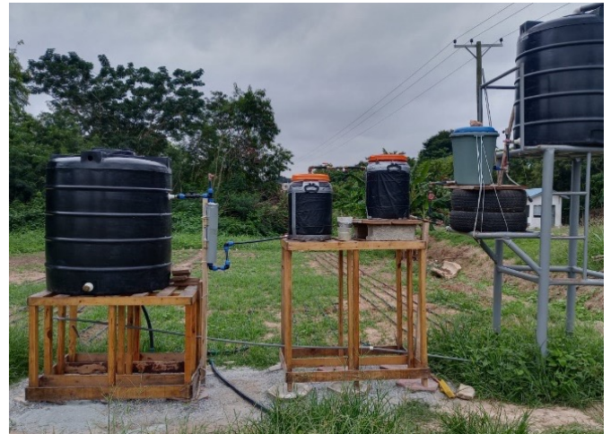
Use of Biochar filters for purifying water for lettuce farming.
