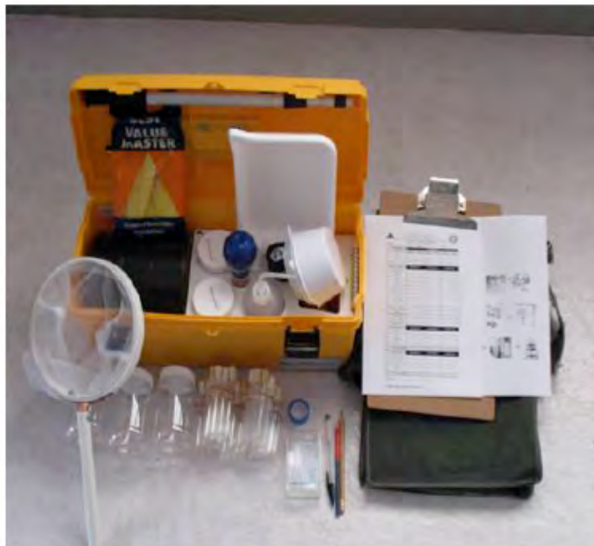
Fig. 2. Field equipment and material required for a pupal survey.
